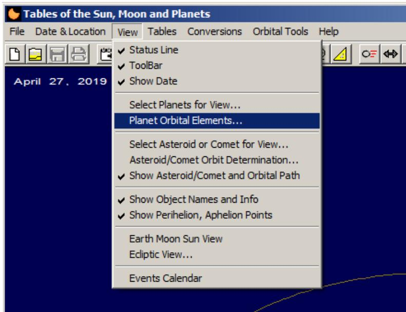
From that dialog box click the **button '?'** at bottom right, and then select the radio button for **Fig. 1** image (see below). The image shows two orbital elements, the **Semi-Major Axis (a)** and the **Eccentricity (e)**.
